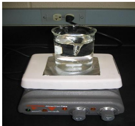
Fig: 4 Magnetic Stirrer-Setting the value of 8 point with 1000 rpm stirring speed and also enhance the direction change for agitation and mixing purpose
