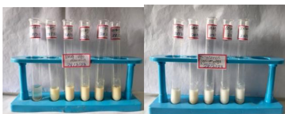
Fig:5 Albumin from eggs procedures 11 test tubes, please. only pour the produced solutions at varied concentrations to 10 test containers, and subsequently add 1 millilitre of dilute saline. The last testing tubes is referred as being the control tube. Add one millilitre of a buffer with phosphate & 1ml of egg albumin that has been taken out of the egg to each tube of testing. After approximately five minutes, everything can be set up on a database lasting a period of time to accumulate OD data.
